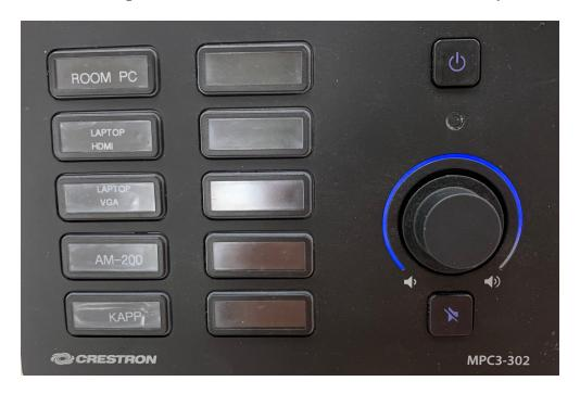
The **Power** button is located in the top right corner, when it is pressed it will power on or off the control panel and the three wall mounted screens.
