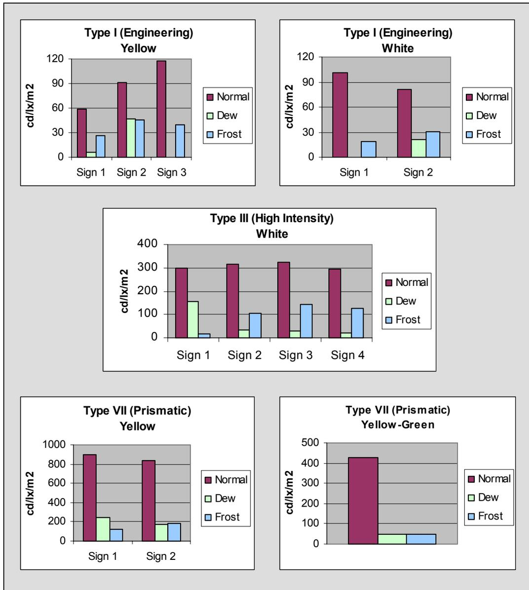
**Figure 9 - Reduction in Retroreflectivity Levels of In-Service Signs Caused by Dew and Frost**
