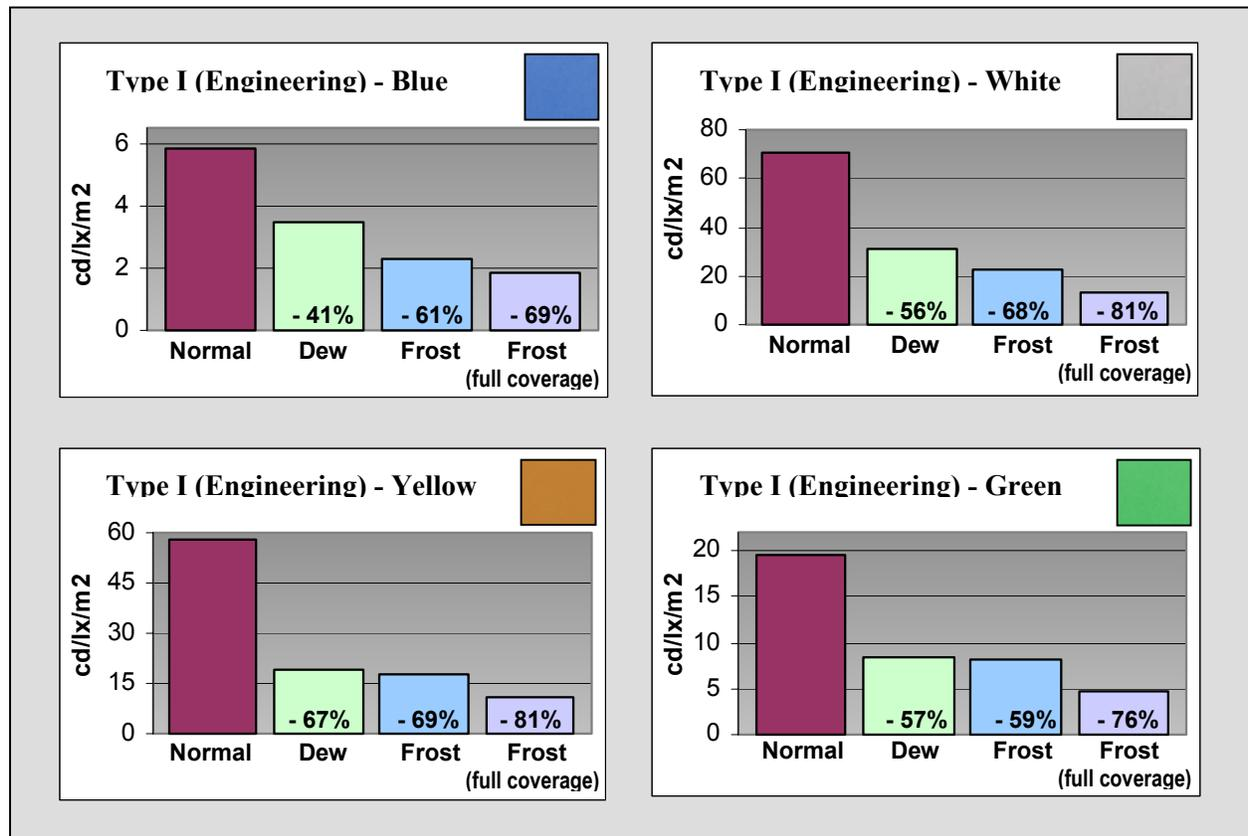
Figure 4a - Reduction in Retroreflectivity Levels Caused by Dew and Frost for Type I (Engineering) Sheeting
