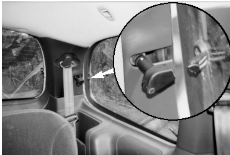
Figure 4: Failure of Side Window Latch
