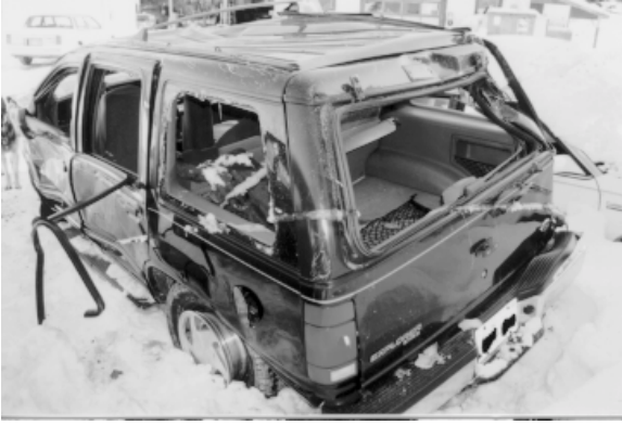
Figure 2: Loss of Side/Rear Glazing
