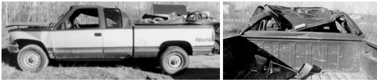
Figure 6: Roof Crush: 1997 Chevrolet Pickup
