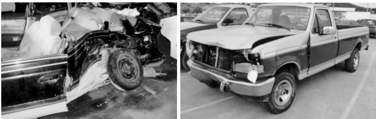
Figure 8: T-type Impact Damage Between Incompatible Vehicles
