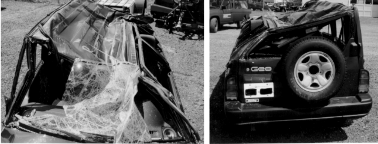
Figure 5: Roof Crush: 1997 Geo Tracker
