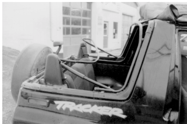
Figure 7: Lack of Protective Roof Structure
