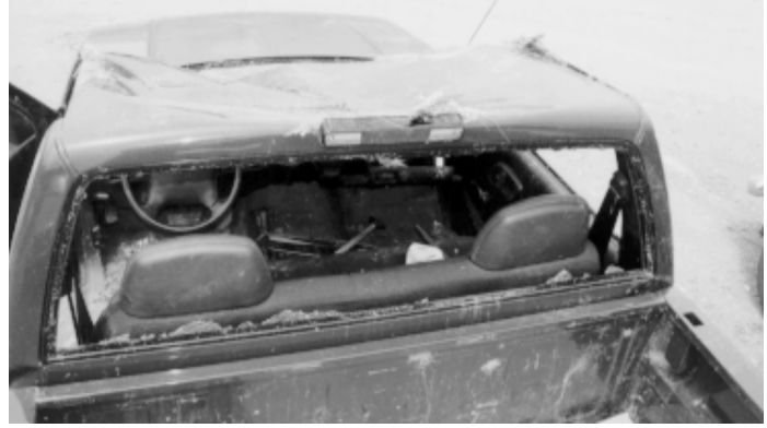
Figure 3: Loss of Rear Glazing
