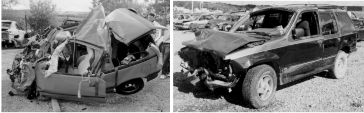
Figure 9: Head-on Impact Damage Between Incompatible Vehicles
