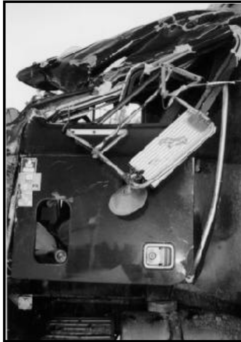
Figure 4: Cab Roof Collapse of Tractor
