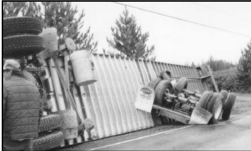
Figure 5: Separation of Tandem Axle Assembly
