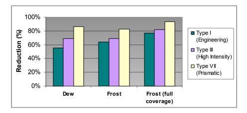
Figure 5 - Reduction in Retroreflectivity Levels by Material Type
