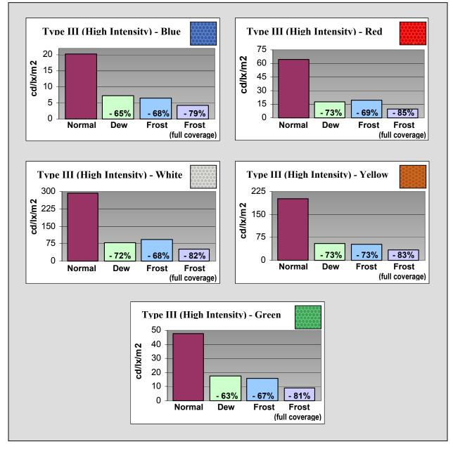
Figure 4b - Reduction in Retroreflectivity Levels Caused by Dew and Frost for Type III (High Intensity) Sheeting
