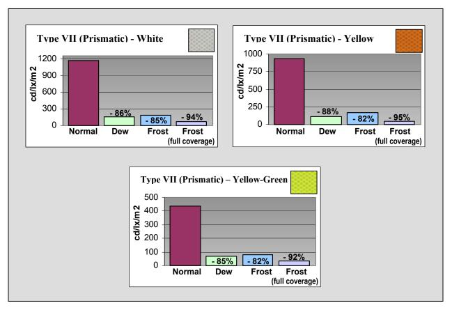
Figure 4c - Reduction in Retroreflectivity Levels Caused by Dew and Frost for Type VII (Prismatic) Sheeting
