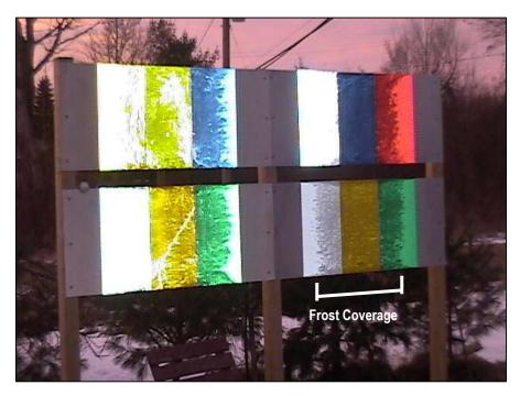
**Figure 7 - Partial Frost Coverage**
