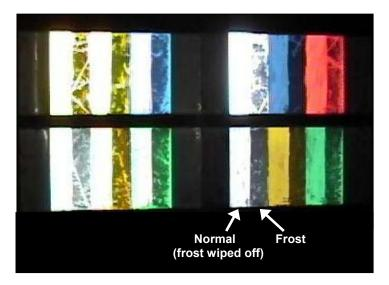
Figure 3 - Test Deck with Frost Present
