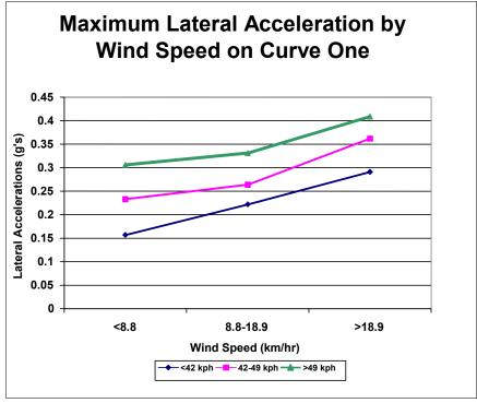
FIGURE 3 Lateral acceleration by wind speed of curve one on the trailer.
