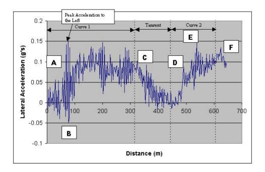
FIGURE 2 Lateral Accelerations vs. Distance on the Ramp.
