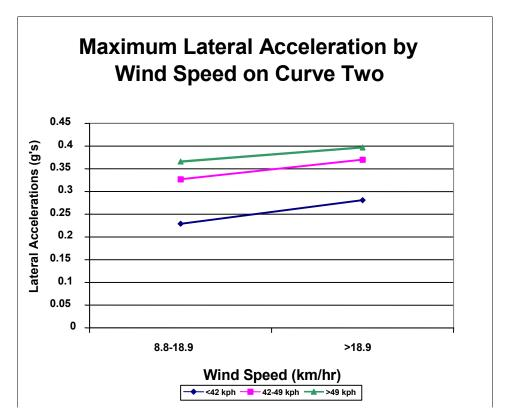
FIGURE 4 Lateral acceleration by wind speed of curve two on the trailer.
