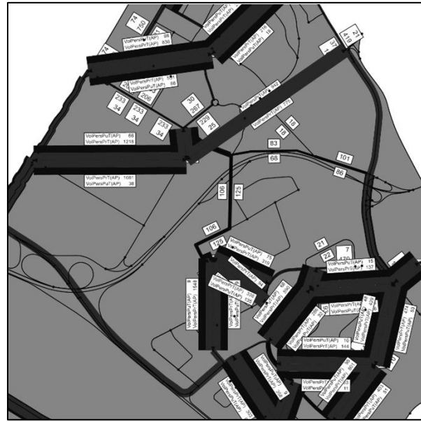
Figure 3: Network after AT link added
