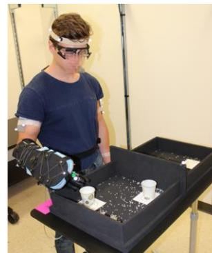
Figure 6: SSMP in use during cup transfer task, with the motion capture and eye tracking setup.
