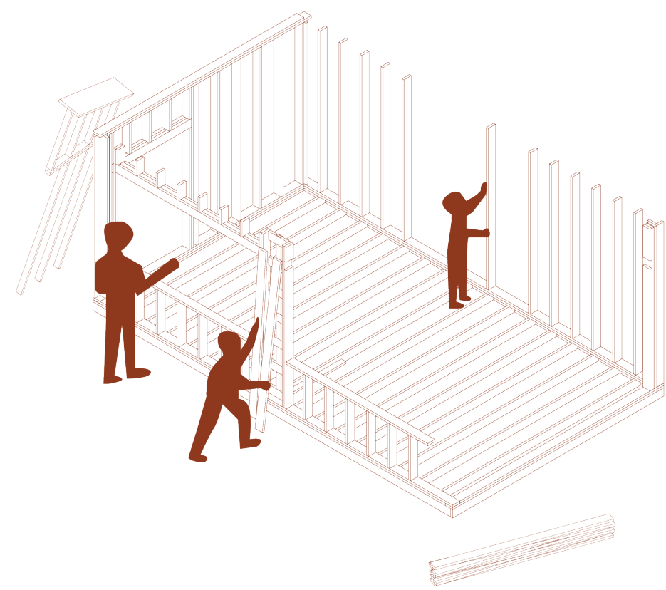
DAY 0 Step 1: Studs for exterior, interior walls and floor
