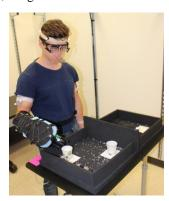
Figure 6: SSMP in use during cup transfer task, with the motion capture and eye tracking setup.
