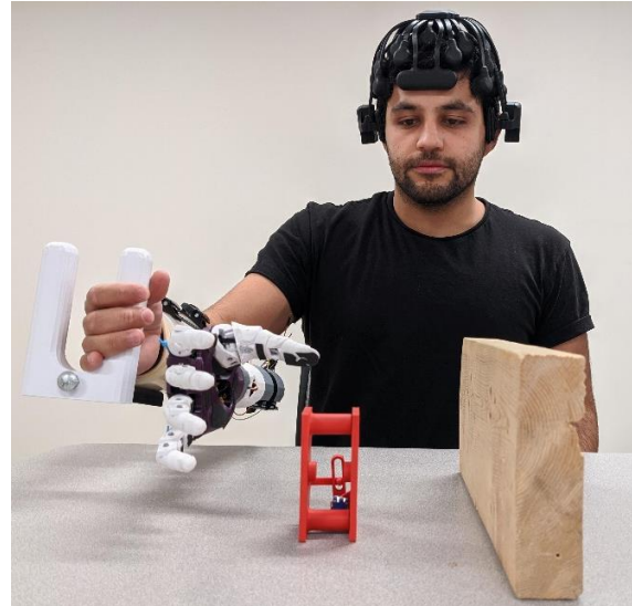
Figure 1. Experimental set-up displaying the custom prosthesis simulator and the dry-wireless EEG system. During experiments, the user's hand and arm are visually occluded.
