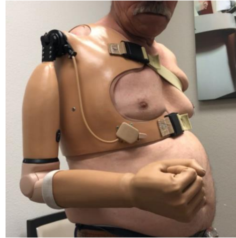
Figure 3: Definitive prosthesis inclusive of pattern recognition control of an Espire Elbow, MC wrist rotator and BeBionic Hand.
