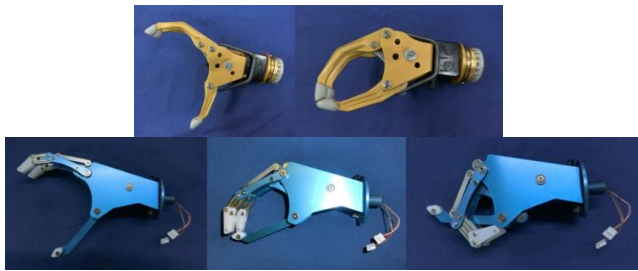
Figure 1: DMC (top) and TRX (bottom) hand's full open/close state
