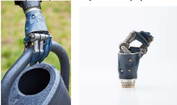
Figure 7: MyHand Power Grip and Fist Grip
