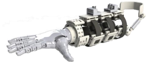
Figure 1: Overview of the 3D-printable MAPP with a HANDI-hand attached to it [2].
