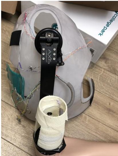
Figure 2: Dynamic test socket with 8 electrodes positioned over targeted muscle sites
