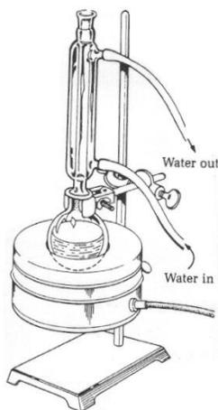
4. Heat the flask to boiling for 30 minutes. The Thermowell Controller should be around 45 and the stir knob should be around 3 on the stirrer/hotplate.
