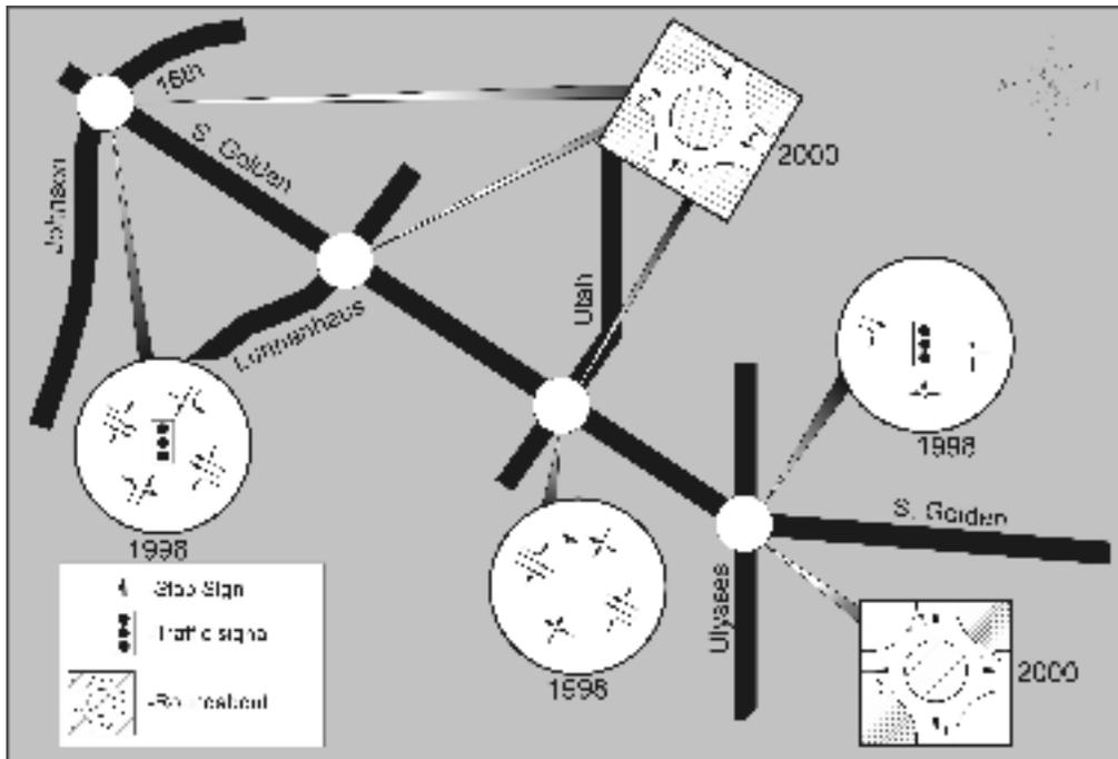
**Figure 1 - Lane Configurations and Traffic Control**
